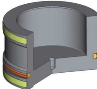
One point Sealing System (≤ Ø180mm)
